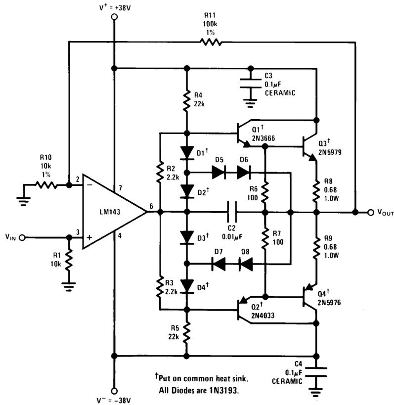
† The 38V supplies allow for a 5% voltage tolerance. All resistors are 1/2 watt, except as noted.
