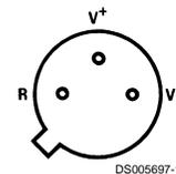
V<sup>-</sup> Pin is electrically connected to case.
