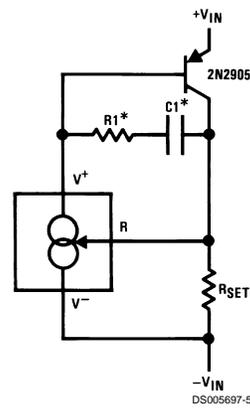
\*Select  $R_1$  and  $C_1$  for optimum stability
