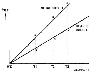
FIGURE 2. Gain Adjustment
