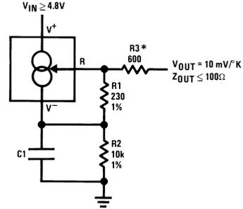
\*Output impedance of the LM134 at the "R" pin is approximately
