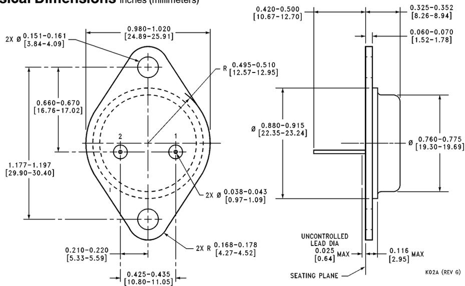
**Steel TO-3 Metal Can Package (K STEEL)**
