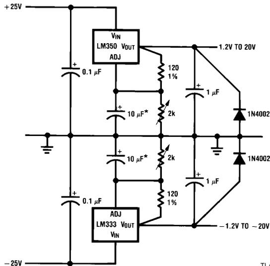
\*The 10 µF capacitors are optional to improve ripple rejection.
