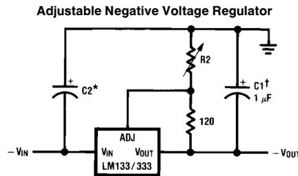
$$-V_{OUT} = -1.25V \left( 1 + \frac{R_2}{120\Omega} \right) + (-I_{ADJ} \times R_2)$$
