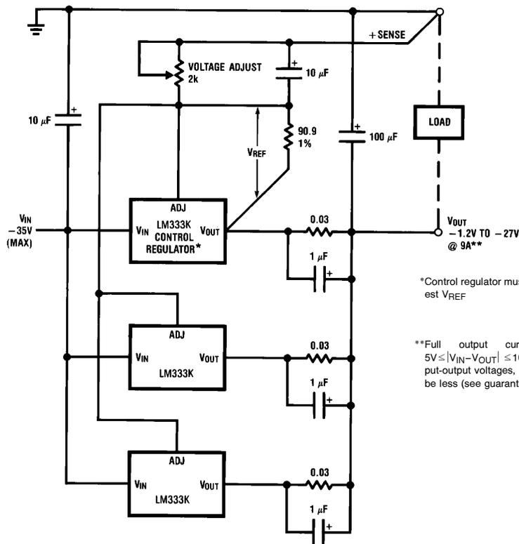
\*Control regulator must have the largest  $V_{REF}$
