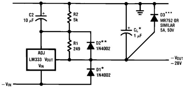
\*When  $C_L$  is larger than  $20 \mu\text{F}$ , D1 protects the LM133 in case the input supply is shorted.
