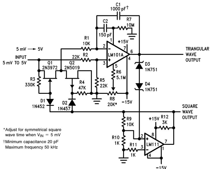
\*Adjust for symmetrical square wave time when  $V_{IN} = 5 \text{ mV}$
