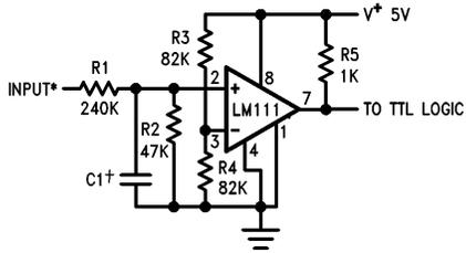
\*Values shown are for a 0 to 30V logic swing and a 15V threshold.
