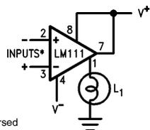
\*Input polarity is reversed when using pin 1 as output.
