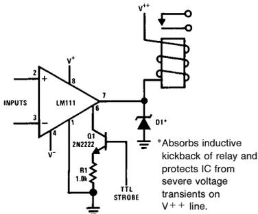
\*Absorbs inductive kickback of relay and protects IC from severe voltage transients on V+ line.
