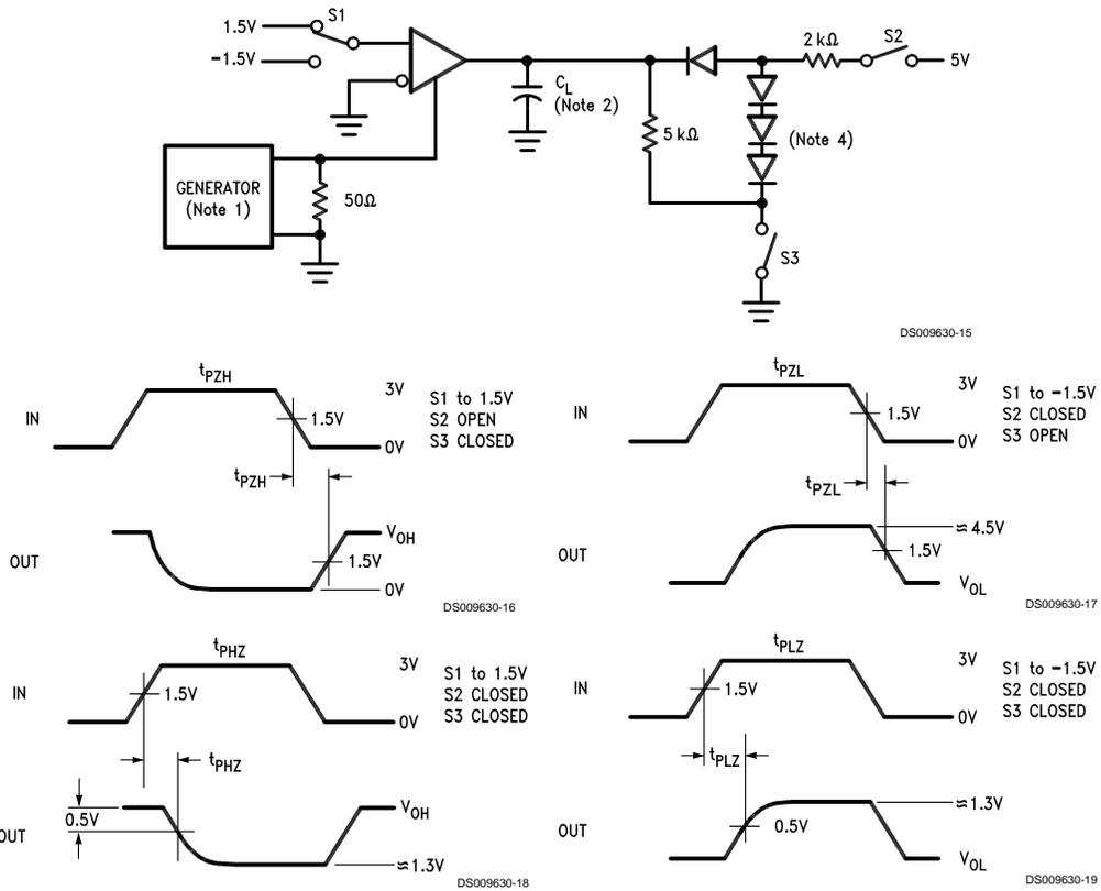
**Note 11:** The input pulse is supplied by a generator having the following characteristics: PRR = 1.0 MHz, 50% duty cycle,  $t_r \leq 6.0$  ns,  $Z_0 = 50\Omega$ .
