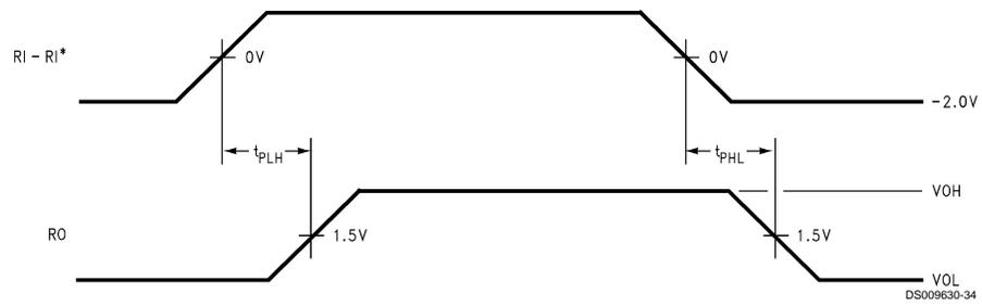
FIGURE 15. Typical Curve Receiver Propagation Delay Timing
