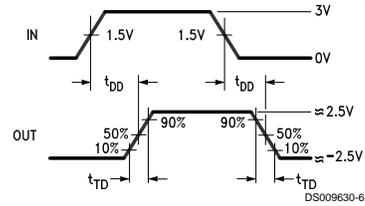
FIGURE 4. Driver Differential Output Delay and Transition Times
