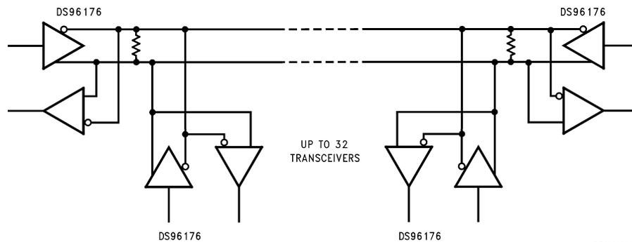
**Note:** The line length should be terminated at both ends of its characteristic impedance. Stub lengths off the main line should be kept as short as possible.
