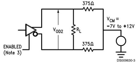
FIGURE 2. Driver  $V_{OD}$  with Varying Common Mode Voltage
