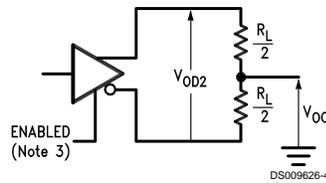
FIGURE 1. Differential and Common Mode Output Voltage
