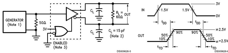
FIGURE 2. Differential Output Delay and Transition Times
