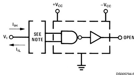
When testing  $I_{IH}$ , the other input is at 3V; when testing  $I_{IL}$ , the other input is open.
