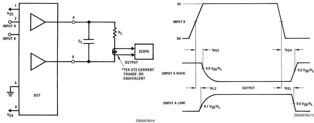
FIGURE 4. TRI-STATE Delays
