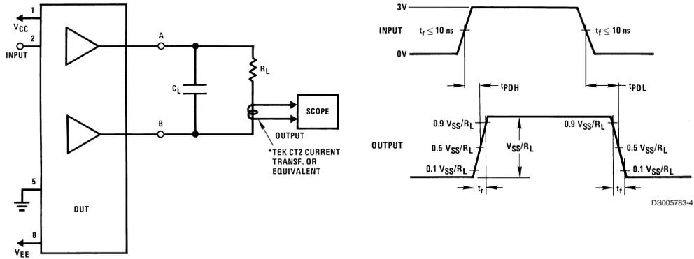
FIGURE 1. Differential Connection
