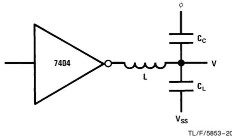
**FIGURE 5. Clock Coupling**
