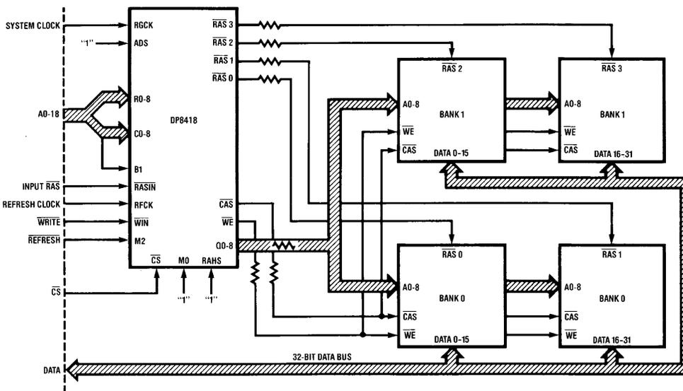
FIGURE 7c. Typical Application of DP8418 Using Modes 5 and 1
