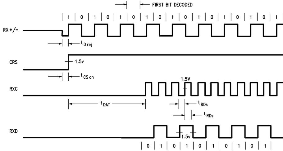
FIGURE 7. Receive Timing - Start of Packet
