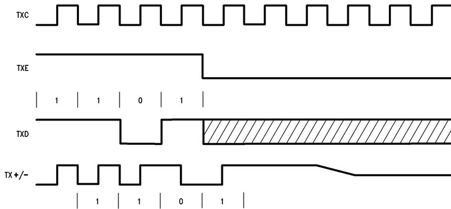
FIGURE 6. Transmit Timing - End of Transmission (last bit = 1)
