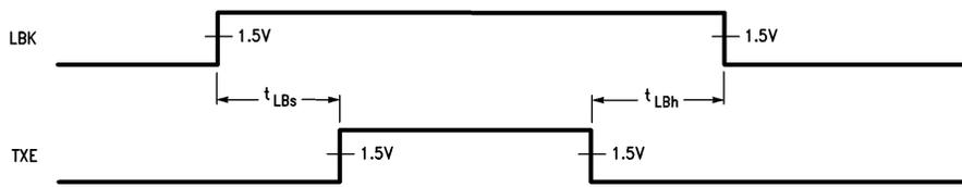
FIGURE 11. Loopback Timing
