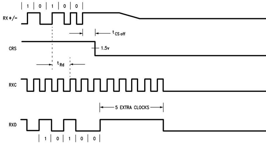
FIGURE 8. Receive Timing - End of Packet (last bit = 0)
