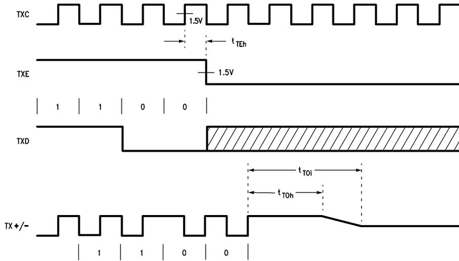
FIGURE 5. Transmit Timing - End of Transmission (last bit = 0)
