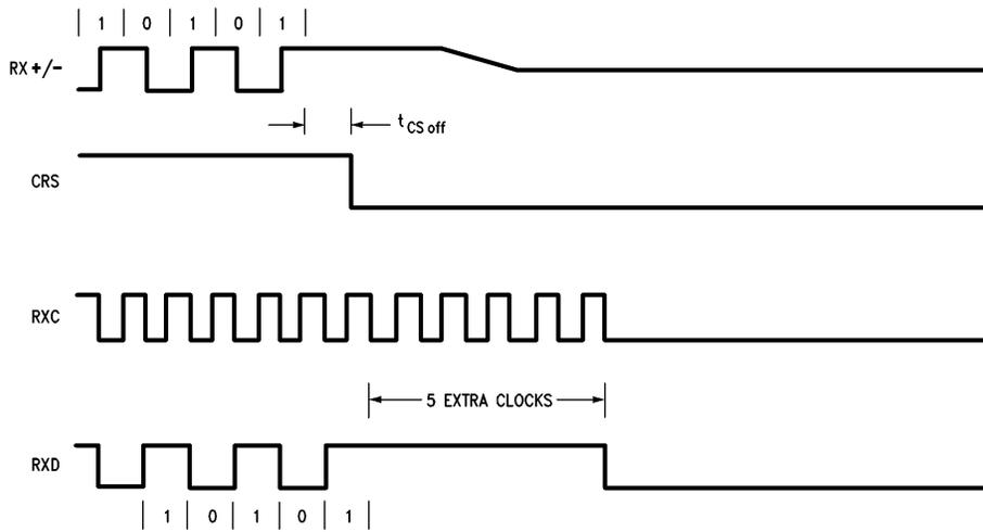
FIGURE 9. Receive Timing - End of Packet (last bit = 1)
