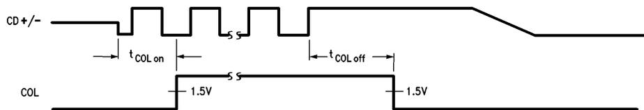
FIGURE 10. Collision Timing
