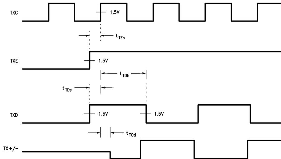
FIGURE 4. Transmit Timing - Start of Transmission
