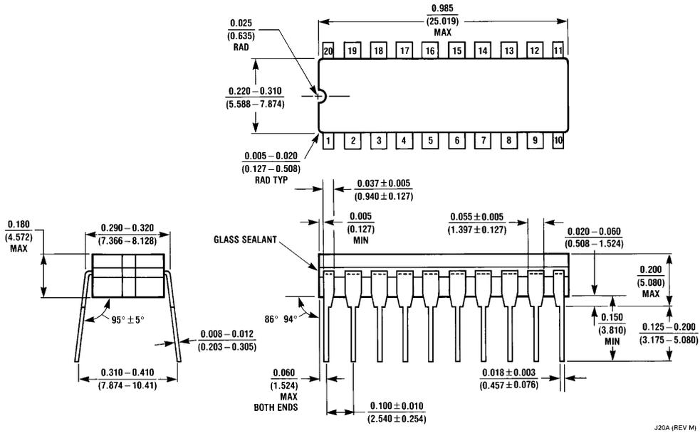
**20-Lead Ceramic Dual-In-Line Package (D)**
