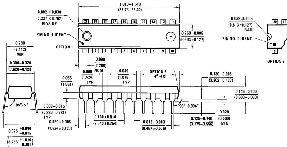
**20-Lead (0.300" Wide) Molded Dual-In-Line Package (P)
