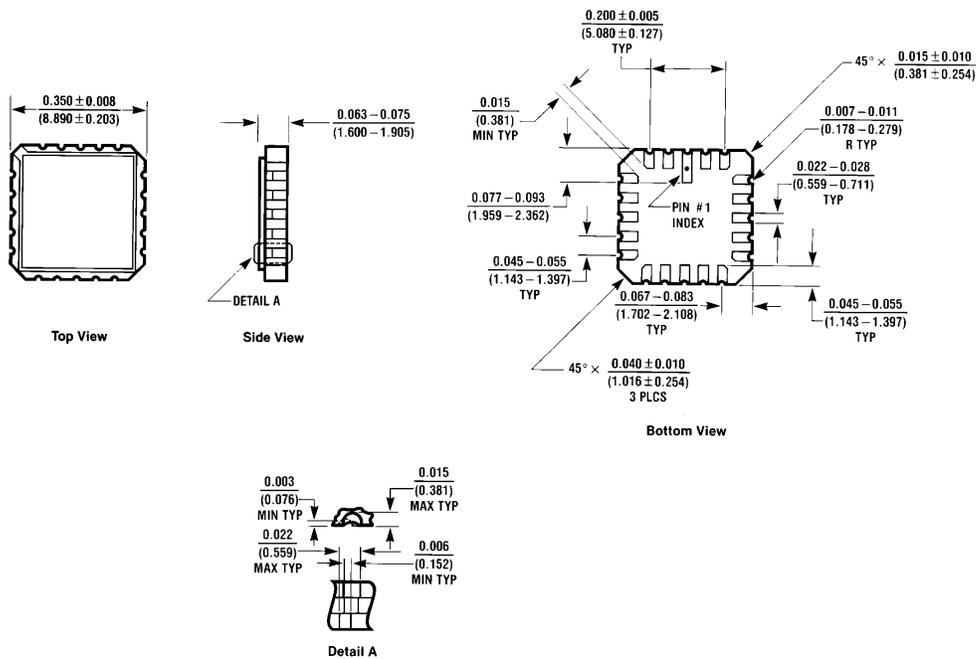
**20-Lead Ceramic Leadless Chip Carrier (L)**
