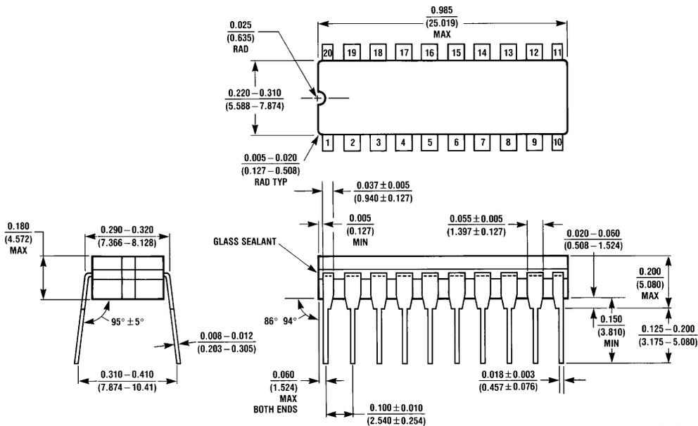
**20-Lead Ceramic Dual-In-Line Package (D)**
