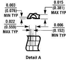
**20-Lead Ceramic Leadless Chip Carrier (L)**
