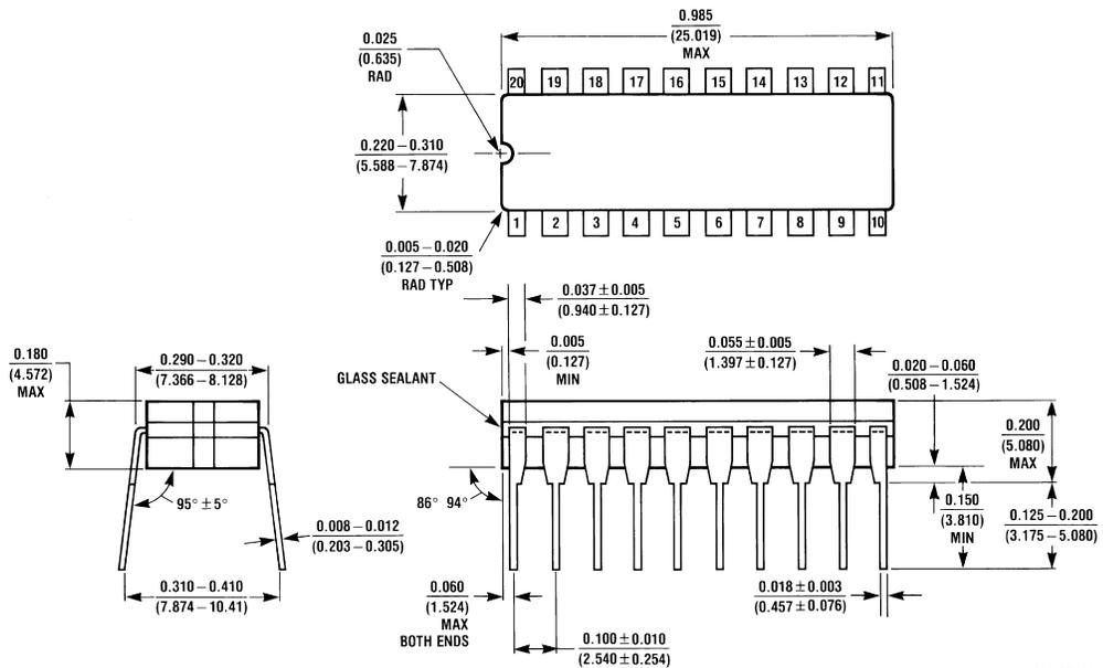
**20-Lead Ceramic Dual-In-Line Package (D)**
