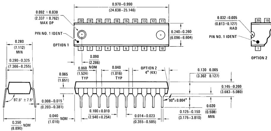
**20-Lead Plastic Dual-In-Line Package (P)**
