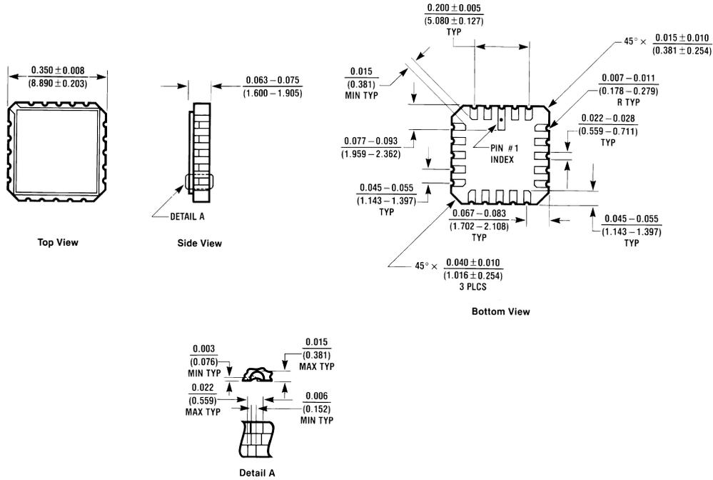
**20-Lead Ceramic Leadless Chip Carrier (L)
