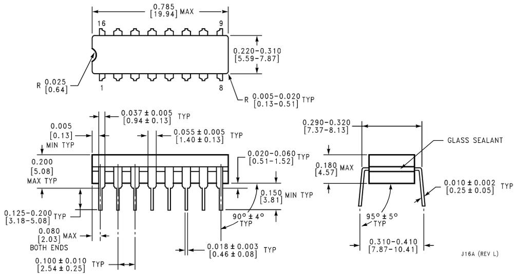
**16-Lead Ceramic Dual-In-Line Package (D)
