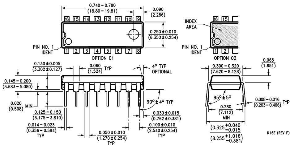
**16-Lead Molded Dual-In-Line Package (N)**
