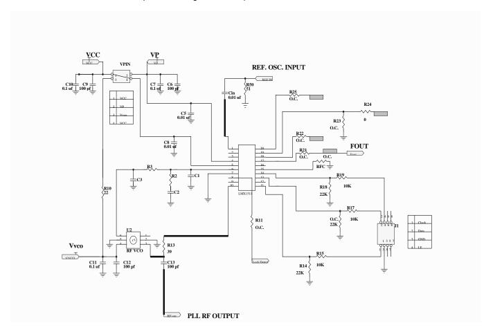
Figure 1 - Schematic for the LMX1511 Evaluation Board
