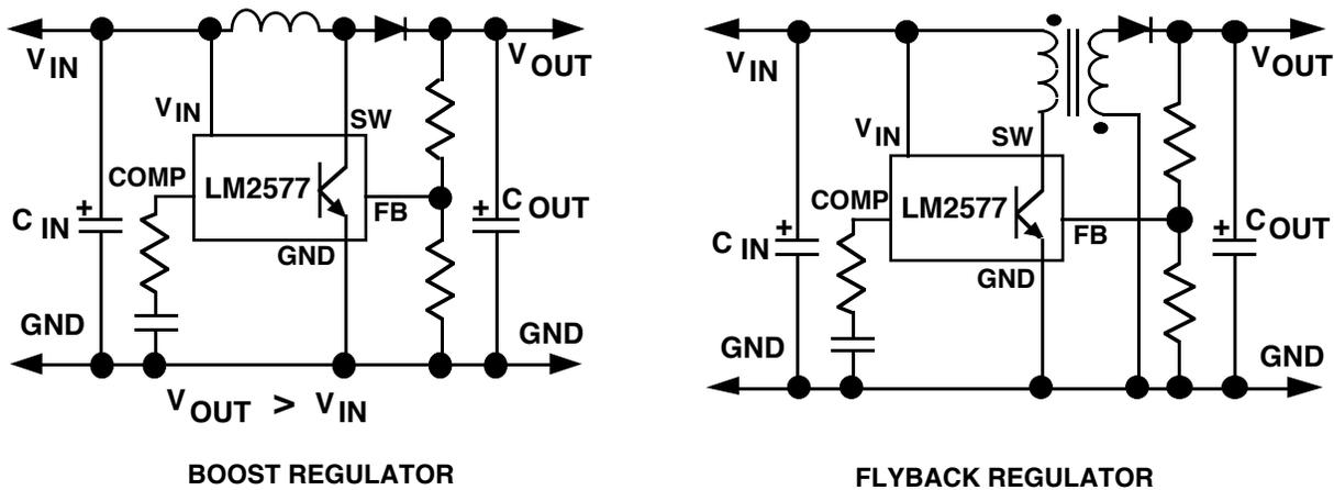
FIGURE 49. BASIC APPLICATION CIRCUITS FOR THE LM2577
