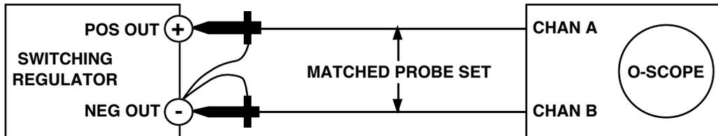
NOTE: INVERT CHANNEL B AND ADD TO CHANNEL A TO REMOVE COMMON-MODE SIGNAL
