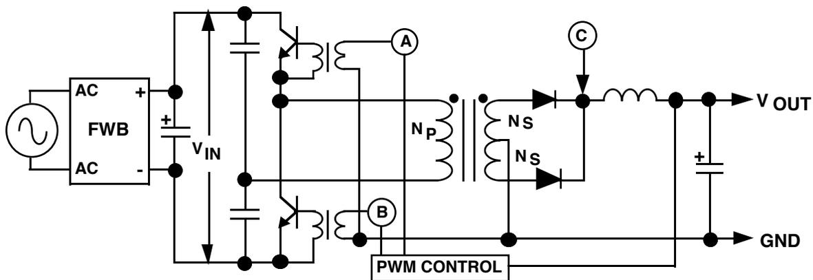
FIGURE 37. HALF-BRIDGE CONVERTER
