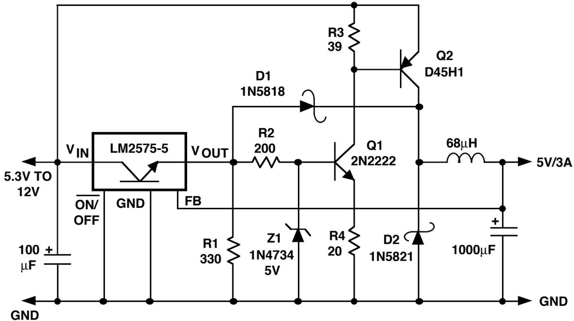
FIGURE 55. LOW-DROPOUT 5V/3A REGULATOR
