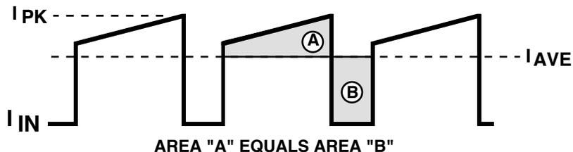
FIGURE 46. AVERAGE VALUE OF TYPICAL INPUT CURRENT WAVEFORM
