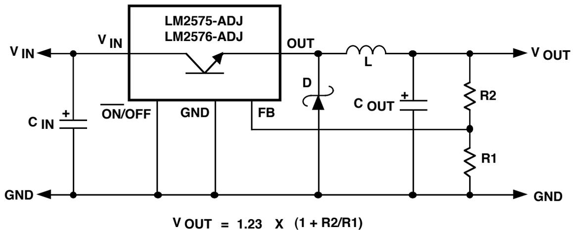
FIGURE 53. LM2575 AND LM2576 BUCK REGULATOR APPLICATION
