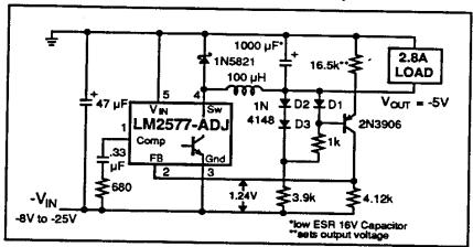
used in a non standard configuration to provide a negative buck regulator function. The 3 Amp IC switch current rating allows the regulator circuit to provide a guaranteed 2.8 Amps of load current when the circuit is operating in the continuous mode.
