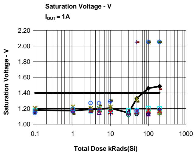
Note: N = 12,  $V_{IN} = 12V$ ,  $I_{LOAD} = 200mA$  unless otherwise stated. MDS - MNLM1575-X-ADJ limits are shown.
