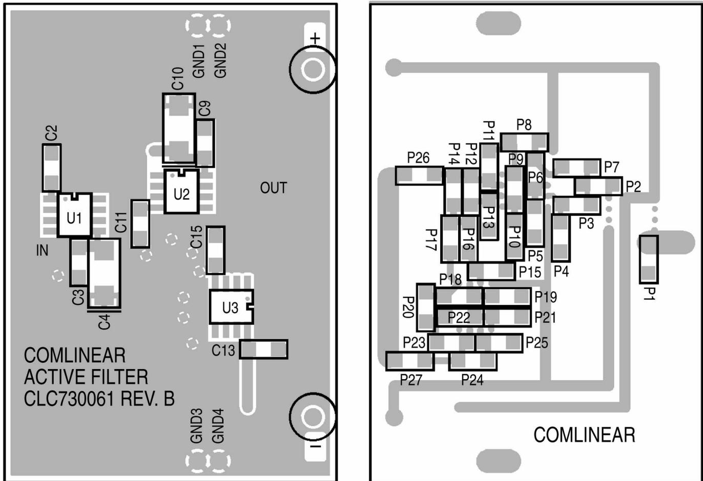
Figure 7: Top & Bottom Views of Active Filter Evaluation Board
