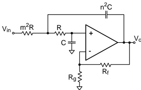
**Figure 8: 2 Pole Sallen-Key Low Pass Filter with Unequal Capacitors**
