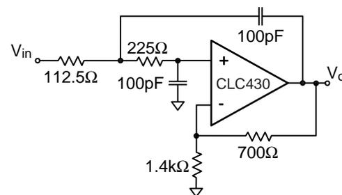
**Figure 2: Example of Low Pass Filter**
