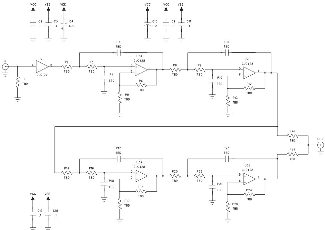
**Figure 6: Schematic for Active Filter Board**
