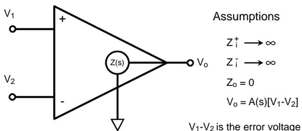
**Figure 1: Voltage Feedback Op Amp**
