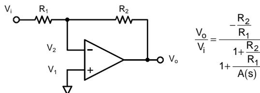
**Figure 2: Voltage Feedback Op Amp Inverting Gain**
