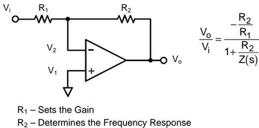
**Figure 5: Current Feedback Op Amp Inverting Gain**
