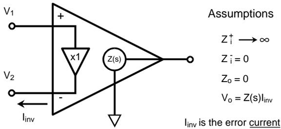
**Figure 4: Current Feedback Op Amp**
