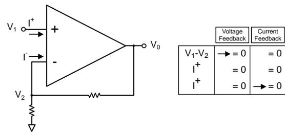
**Figure 9: Op Amp Comparison Closed-Loop Operation**
