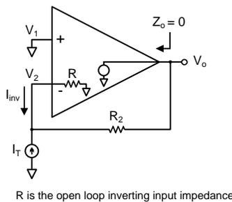
**Figure 7: Closed-Loop Inverting Input Impedance**
