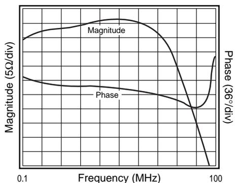
Figure 4a: Input Impedance
