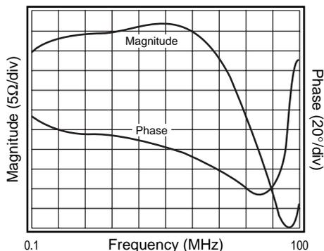
**Figure 7a: Input Impedance**
