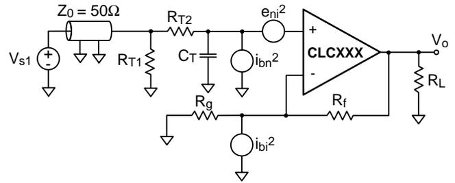
Figure 2: Non-Inverting Gain Amplifier
