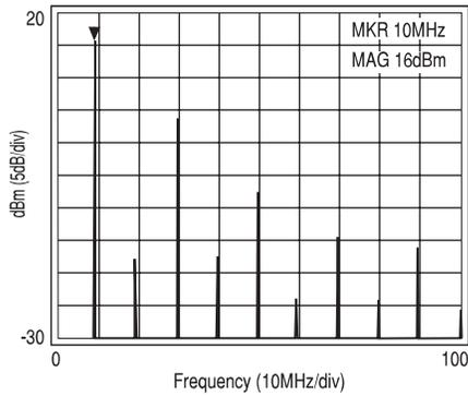
**Figure 12b: Output Spectrum at 10MHz -1dB Compression**
