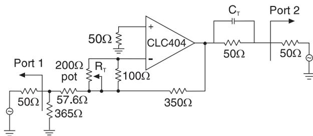
Figure 9A: Inverting Reverse Isolation Test Circuit
