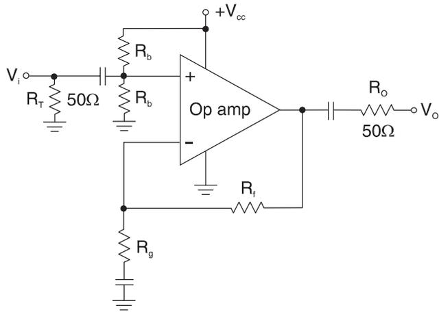
**Figure 4a: Single Supply, Non-Inverting Op Amp Operation**
