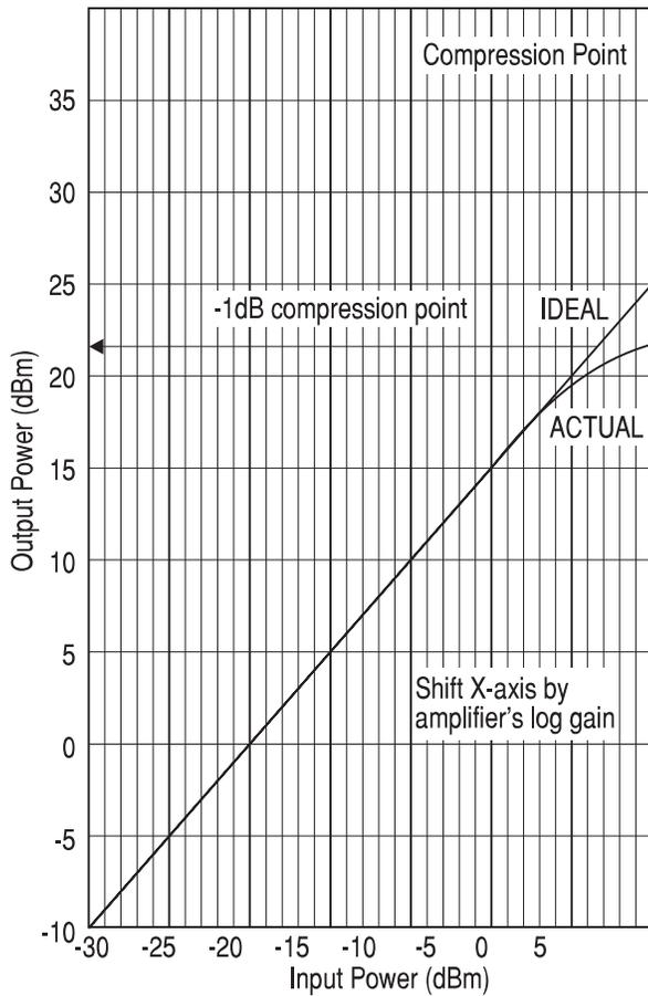
**Figure 10: Illustration of -1dB Compression**
