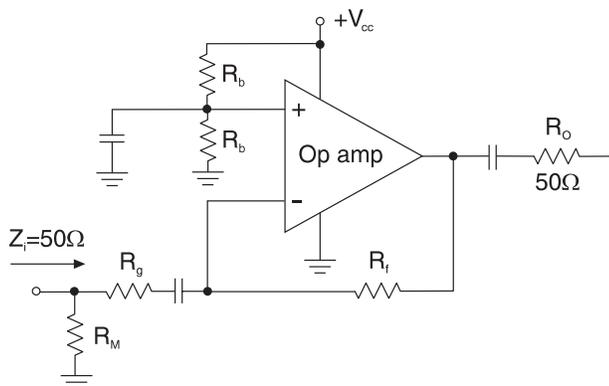
**Figure 4B: Single Supply, Inverting Op Amp Operation**
