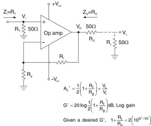
**Figure 2A: Non-Inverting Op Amp Configured for RF Application**
