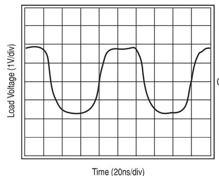
**Figure 12A: Output Waveform at 10MHz -1dB Compression**
