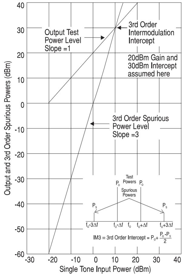
**Figure 14: Output and 3rd Order Spurious Power vs. Input Power**
