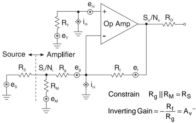
**Figure 21: Inverting Op Amp Noise Figure Analysis**
