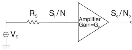
$$\text{Noise Figure} = \text{NF} = 10 \log \left[ \frac{S_i / N_i}{S_o / N_o} \right] = 10 \log \left[ \frac{S_i N_o}{S_o N_i} \right]$$
