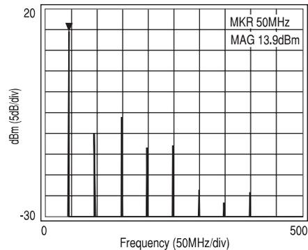
**Figure 13B: Measured Output Spectrum at 50MHz -1dB Compression**
