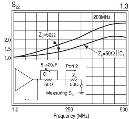
**Figure 6: Measuring and Tuning CLC404 Output VSWR**
