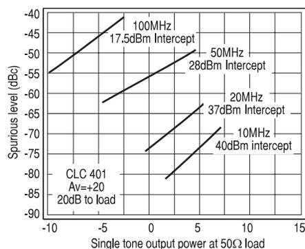
**Figure 17: Measured 3rd Order Spurious for the CLC401**
