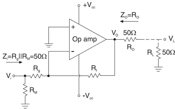
$$A_L^- = -\frac{1}{2} \frac{R_f}{R_g} = \frac{V_L}{V_I}; \text{ neglecting the signal inversion}$$
