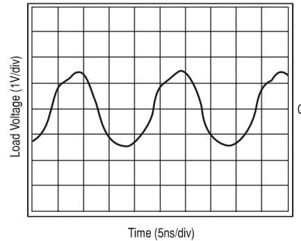
**Figure 13A: Measured Output Waveform at 50MHz -1dB Compression**
