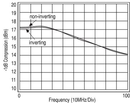
**Figure 11: 1dB Compression for the CLC404**
