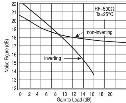
Figure 22: Noise Figure vs. Gain For The CLC404
