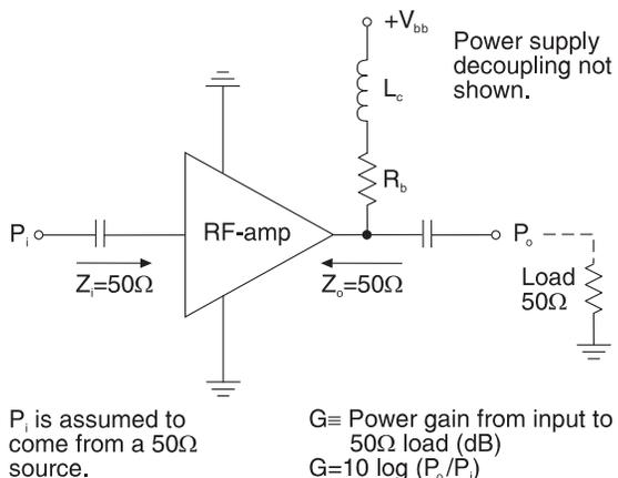
**Figure 1A: Typical RF Amplifier Connection**
