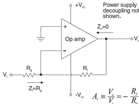
**Figure 1C: Ideal Inverting Op Amp**
