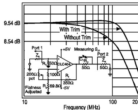
**Figure 8: Measuring and Adjusting the Frequency Response  $S_{21}$**
