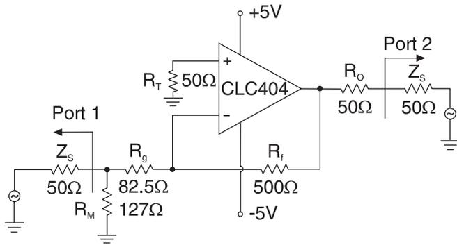
**Figure 5B: Inverting Amplifier S-parameter Test Circuit**
