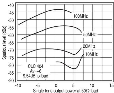
**Figure 16: Measured 3rd Order Spurious for the CLC404**
