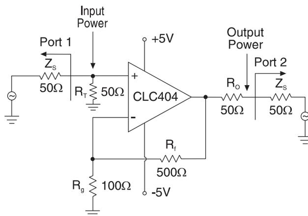
**Figure 5A: Non-inverting Amplifier S-parameter Test Circuit**
