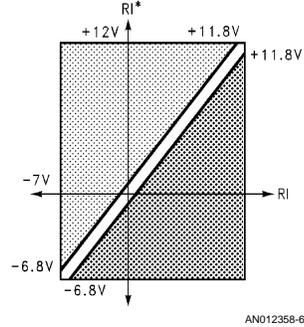
**FIGURE 6. Receiver Input Range**
