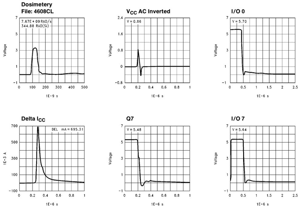
FIGURE 5. 54AC299 Dose Rate Characterization Latchup/Survivability Test, +117°C
