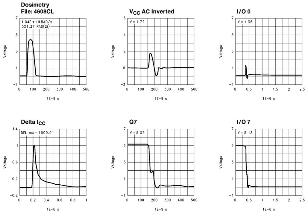
FIGURE 6. Dose Rate Characterization Latchup/Survivability Test, +25°C
