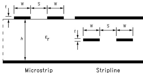
In common practice,  $h$  represents dielectric thickness for microstrip structures and  $b$  that for stripline. For simplicity, the
