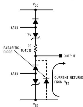
FIGURE 7b. Output Stage Overvoltage Model ( $-V_{EE}$ )
