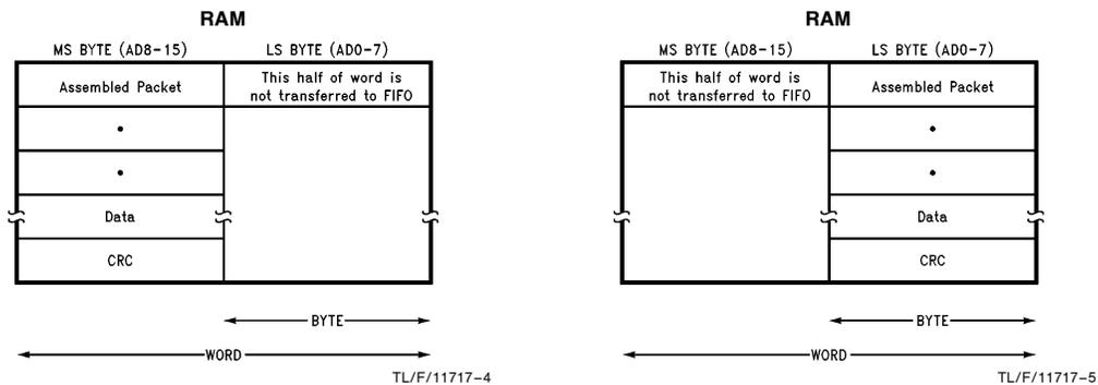
**FIGURE 4. Packet Assembly for Loopback Word Wide Transfers**
