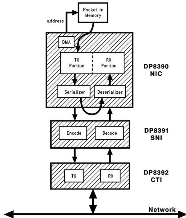
FIGURE 1. Loopback Mode 1: Through the Controller
