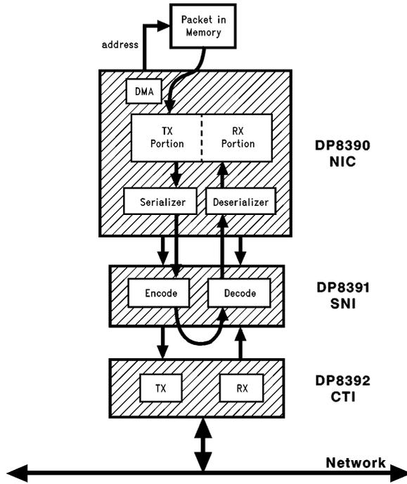
FIGURE 2. Loopback Mode 2: Through the SNI
