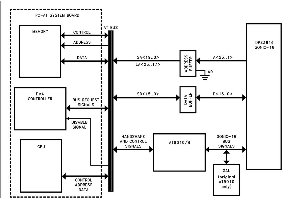
FIGURE 7. Master Logic Block Diagram
