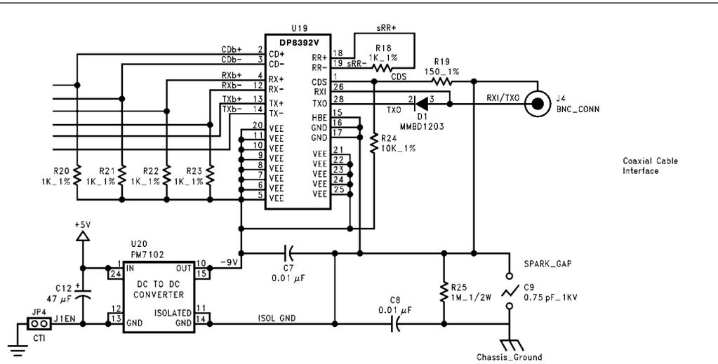
Note: CTI configured for transmit mode collision detection.
