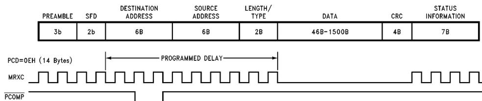
FIGURE 11. Packet Reception Over Management Bus
