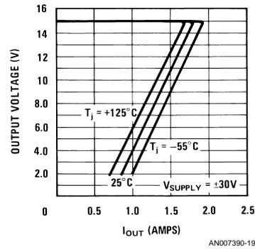
FIGURE 16. Positive Regulator Foldback Current Limiting Characteristics
