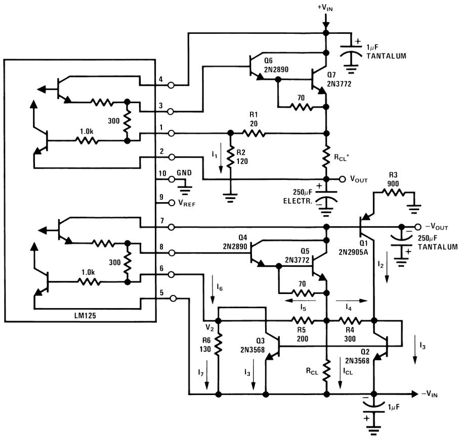
FIGURE 18. 10A Regulator with Foldback Current Limiting
