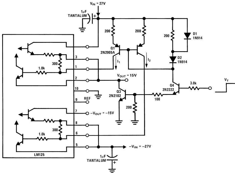
FIGURE 25. Electronic Shutdown for the Basic Regulator
