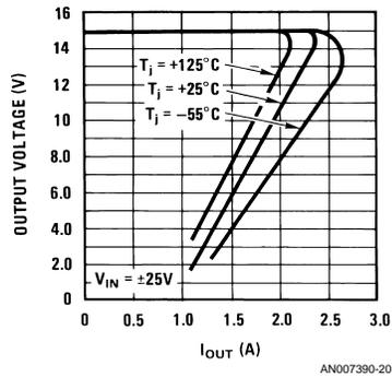
**FIGURE 17. Negative Regulator Foldback Current Limiting Characteristics**
