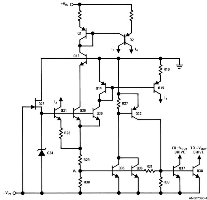
FIGURE 4. Start-up, Biasing and Thermal Shutdown Circuitry
