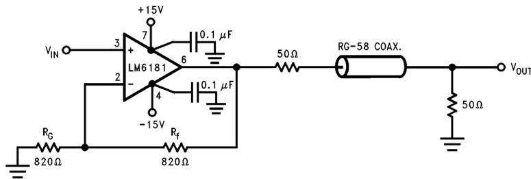
**FIGURE 2. Backmatching of a cable is a clean way of terminating the source to the characteristic impedance. The LM6181 can deliver  $\pm 10\text{V}$  into the resulting dc load of  $100\Omega$ , at 100 MHz, typically.**
