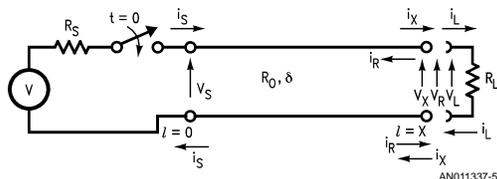
**FIGURE 5. Boundary Conditions at the Line/Load Interface**
