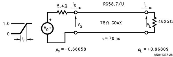
FIGURE 20. Transmission Line Model and Its Lattice Diagram
