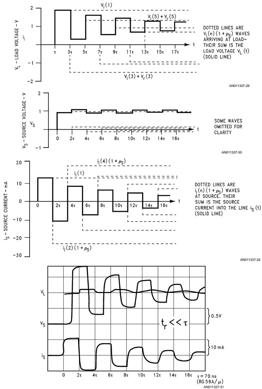
**FIGURE 21. Waveforms for  $t_r = 2 \ll \tau$**
