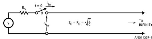
FIGURE 1. Generator Driving an Infinite Transmission Line
