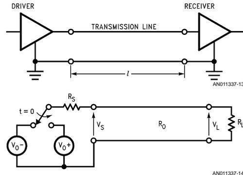
FIGURE 12. Model Used for Lattice Diagram Method
