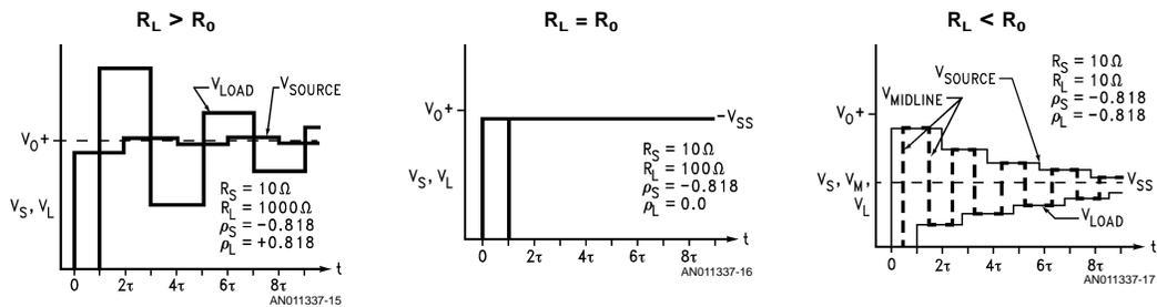
FIGURE 13.  $R_S < R_0$
