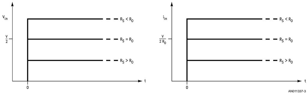
FIGURE 3. Voltage/Current Steps for Three Source Resistances
