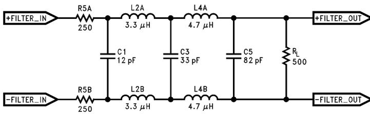
FIGURE 2c. Differential Filter
