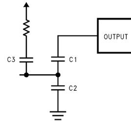
FIGURE 4. Parasitic Capacitance
