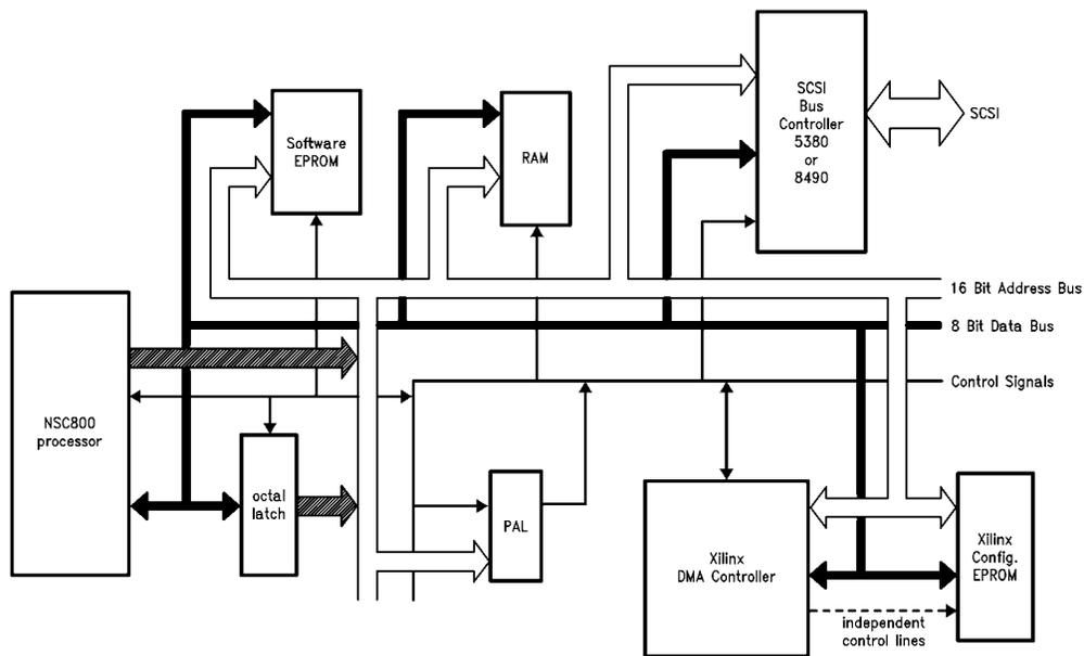
FIGURE 2. Circuit of SCSII Test Board
