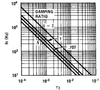
**FIGURE 5. Damping Time Constant vs Natural Frequency**
