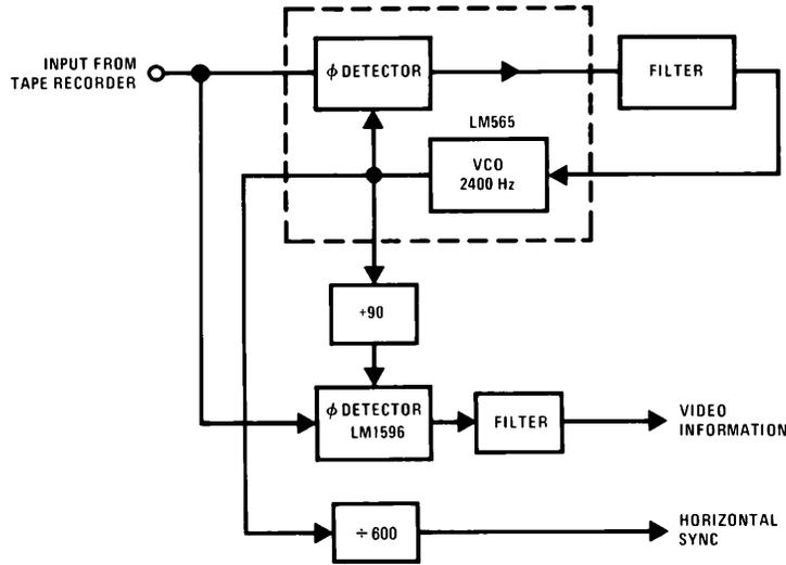
FIGURE 21. Block Diagram of Weather Satellite Demodulator
