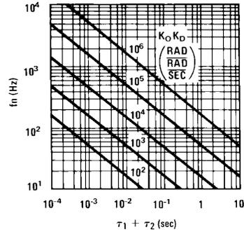
**FIGURE 4. Filter Time Constant vs Natural Frequency**
