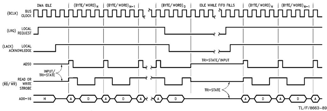
**FIGURE 6.5 (a). Typical Local DMA Burst Transfer Timing**
