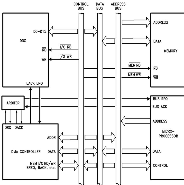
FIGURE 6.7 (a). A Typical External DMA-DDC Interface
