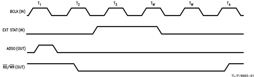
FIGURE 6.6 (b). DMA with External Wait States
