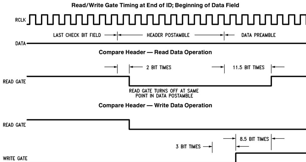
FIGURE 6.20 (b). Read/Write Gate Timing for DDC
