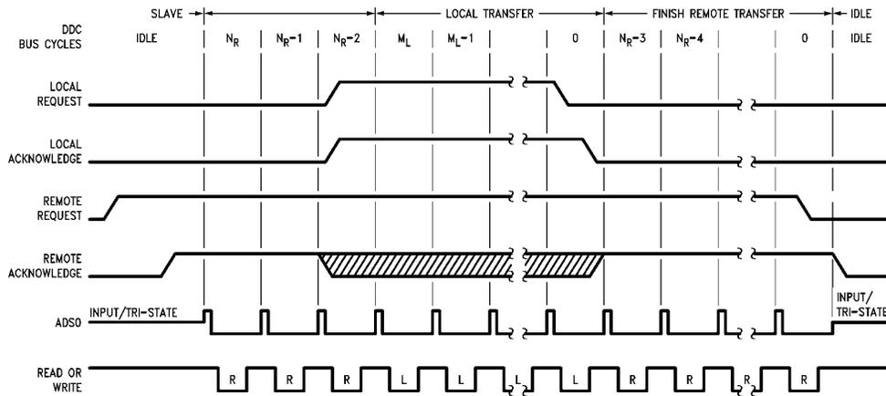
**FIGURE 6.5 (c). Interleaved Remote and Local Transfer Timing**
