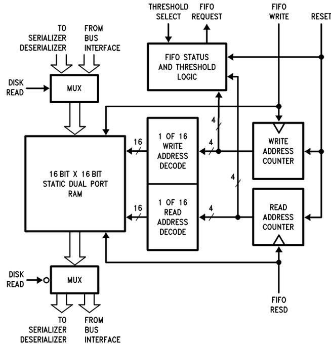
FIGURE 4.4. Simplified Block Diagram of DDC's FIFO
