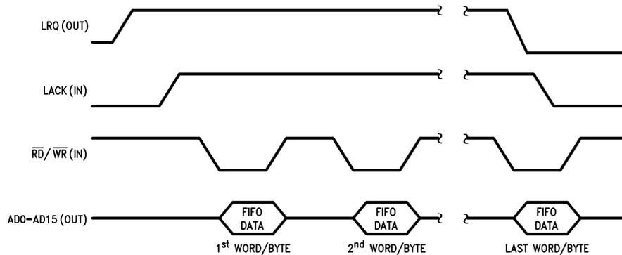
FIGURE 6.7 (b). DDC FIFO Read/Write by External DMA
