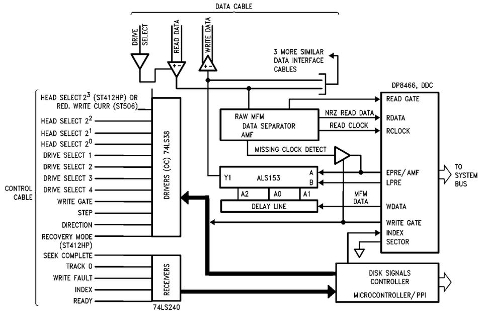
FIGURE 6.14. Disk Data and Control Paths (ST506/ST412HP)
