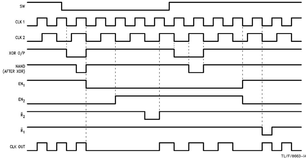
FIGURE 6.27 (b). Timing Diagram for Switching Logic
