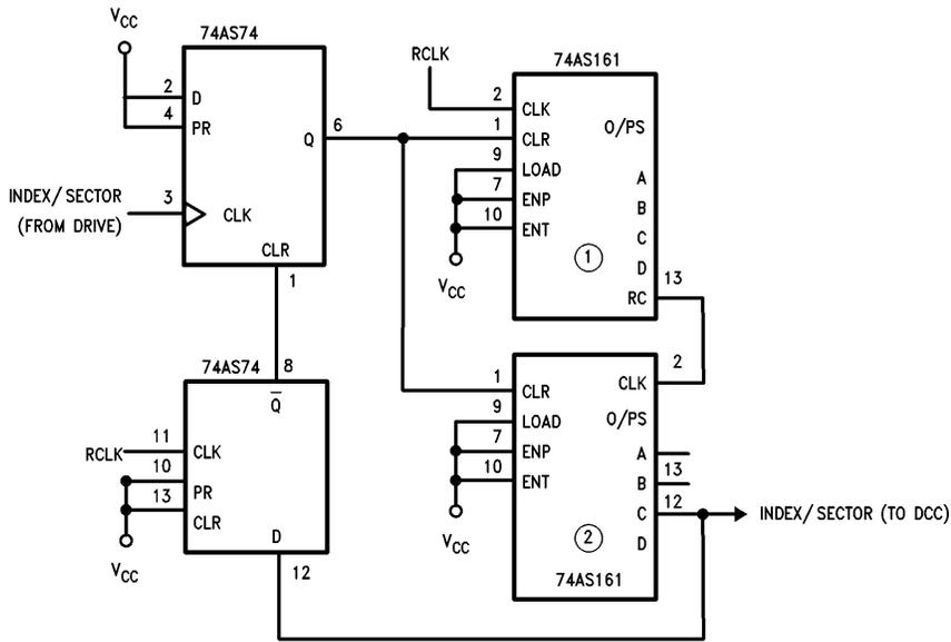
FIGURE 6.28. Logic to Implement Post Index/Sector Gap Field
