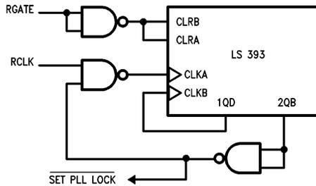
Counter timer using dual 4 bit binary counters cascaded. Count is stopped by decoding bit 2QB which is reached after 32 RCLKS, counter is reset when RGATE is deasserted.
