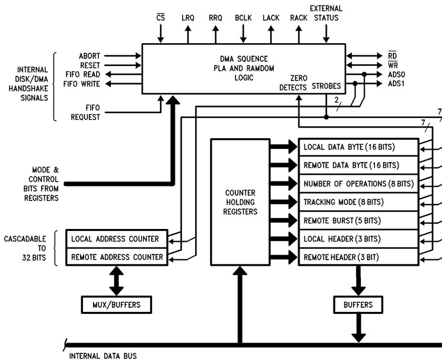
FIGURE 4.6. Block Diagram for Dual/Single Channel DMA Controller
