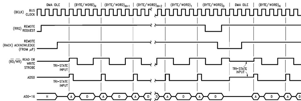
**FIGURE 6.5 (b). Typical Remote DMA Burst Transfer Timing**
