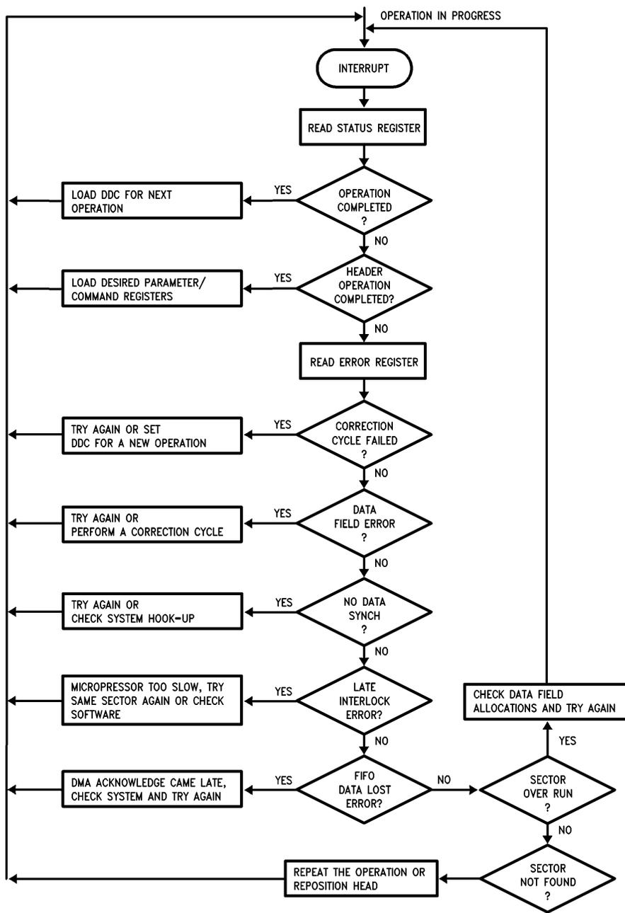
FIGURE 7.22 Interrupt Servicing
