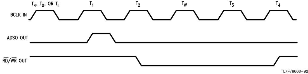
FIGURE 6.6 (a). DMA with Internal Wait States
