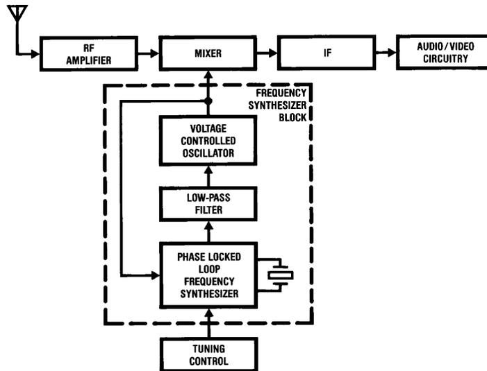
FIGURE 1. Block Diagram of a Digitally Tuned Receiver
