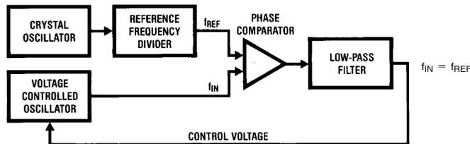
FIGURE 3. Basic Phase-Locked-Loop
