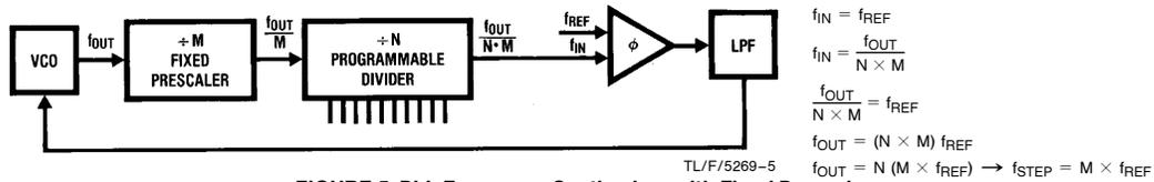
**FIGURE 5. PLL Frequency Synthesizer with Fixed Prescaler**
