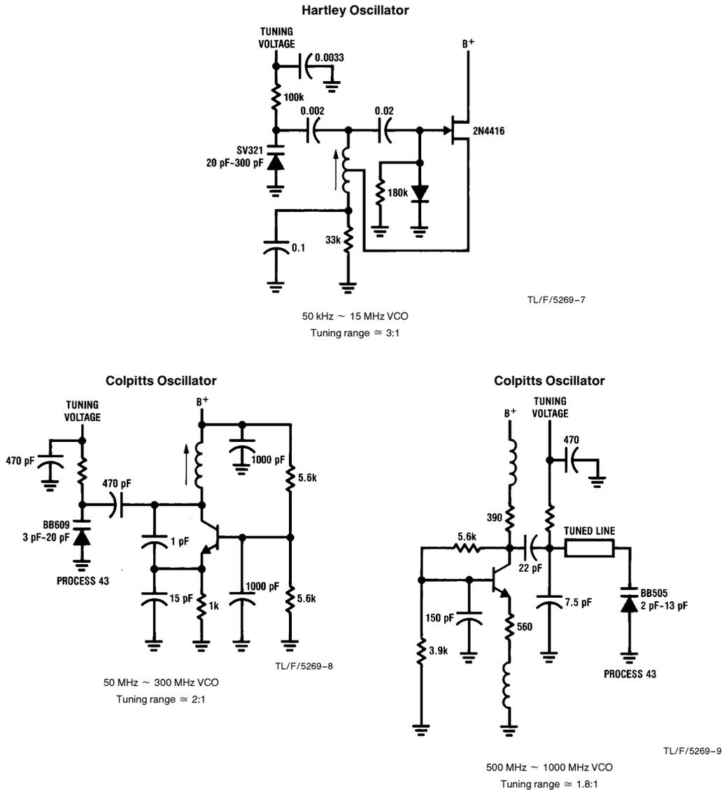
FIGURE 7. Typical VCO Circuits (Typical Values Shown)
