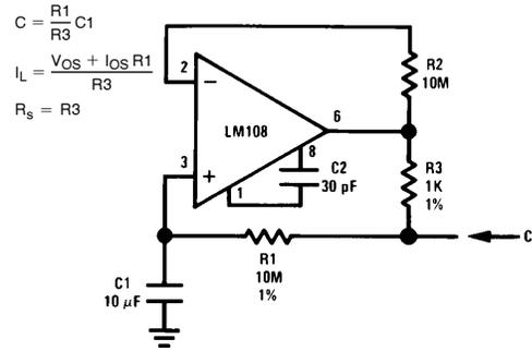
Figure 19. Capacitance multiplier
