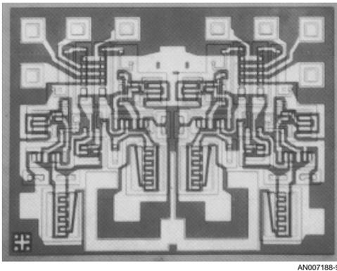
FIGURE 8. Photomicrograph of the DS7830 Dual Line Driver
