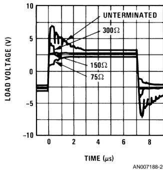
**FIGURE 20. Transmission Line Response with Various Termination Resistances**
