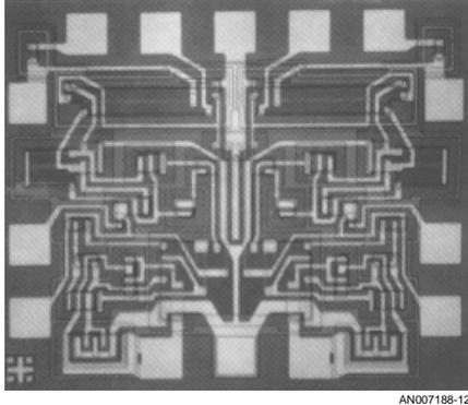
**FIGURE 11. Photomicrograph of the DS7820 Dual Line Receiver**
