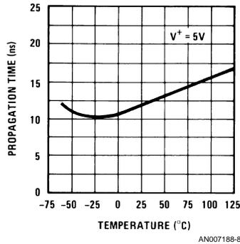
FIGURE 7. Propagation Time as a Function of Temperature
