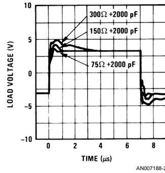
**FIGURE 21. Line Response for Various Termination Resistances with a DC Isolation Capacitor**
