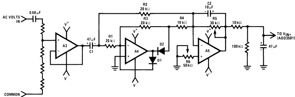
FIGURE 2. AC/DC Converter
