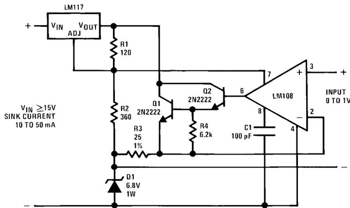
FIGURE 8. 10 mA to 50 mA 2-Wire Current Transmitter
