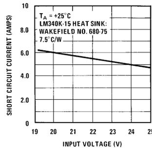
**FIGURE 8. Continuous Short Circuit Current vs Input Voltage**
