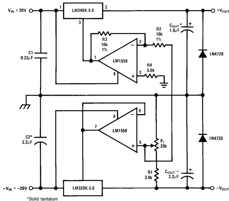
FIGURE 17. Tracking Dual Supply  $\pm 5.0V - \pm 18V$
