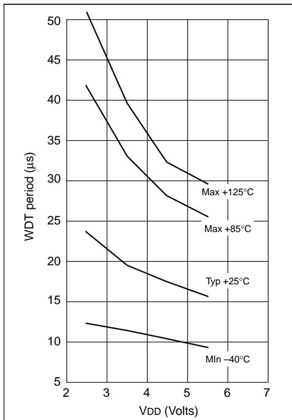
**FIGURE 11-4: SHORT DRT PERIOD VS. V<sub>DD</sub>**
