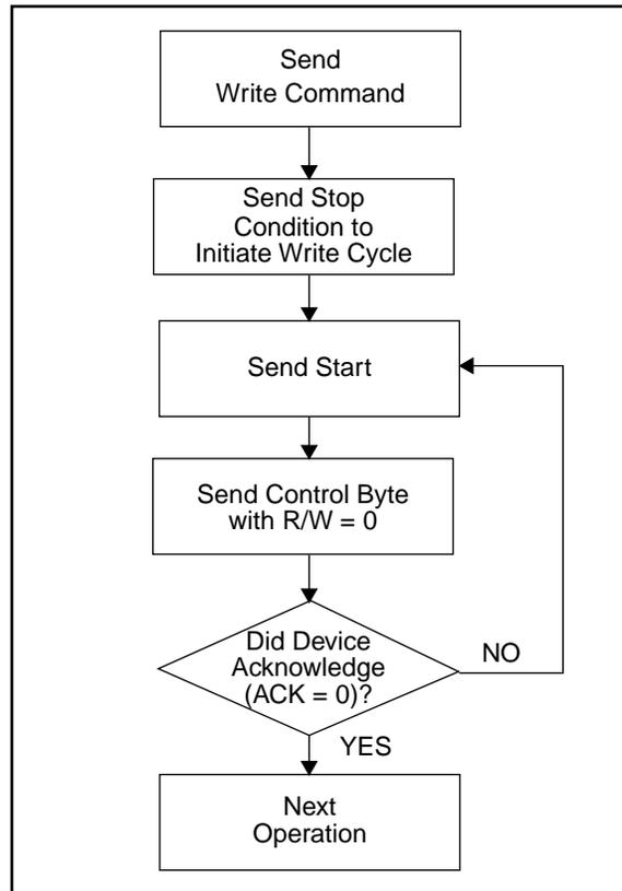
**FIGURE 6-5: BYTE WRITE**
