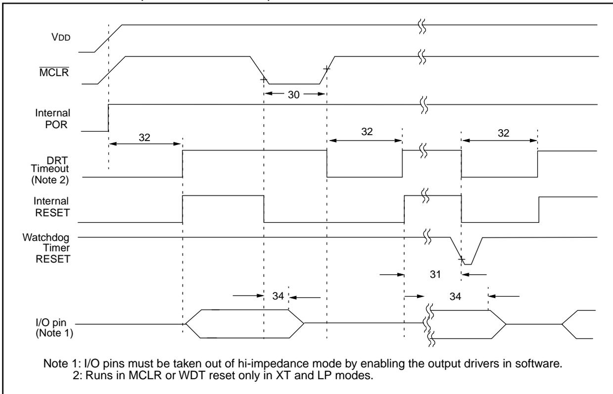
**TABLE 10-5: RESET, WATCHDOG TIMER, AND DEVICE RESET TIMER - PIC12C508/C509**
