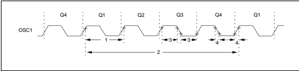
TABLE 10-2: EXTERNAL CLOCK TIMING REQUIREMENTS - PIC12C508/C509
