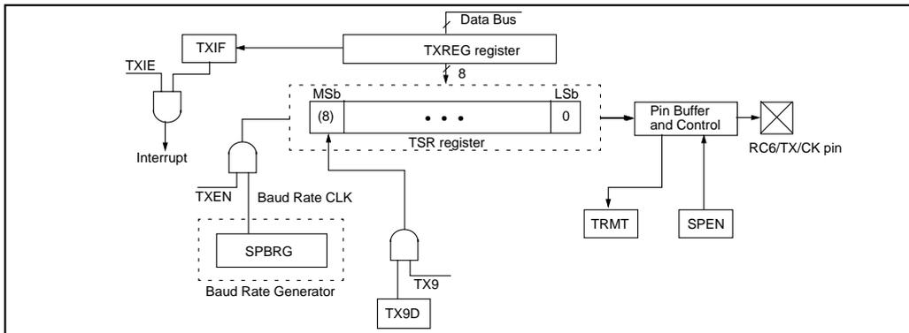
**FIGURE 9-4: ASYNCHRONOUS TRANSMISSION**
