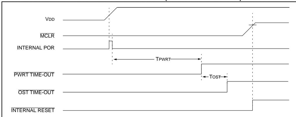
**FIGURE 11-10: SLOW RISE TIME ( $\overline{\text{MCLR}}$  TIED TO  $V_{\text{DD}}$ )**
