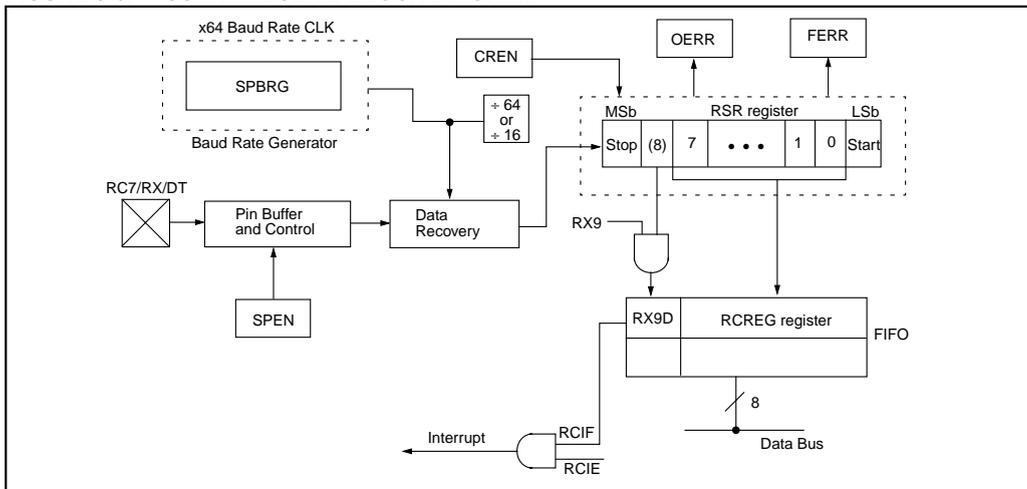
**FIGURE 9-7: ASYNCHRONOUS RECEPTION**
