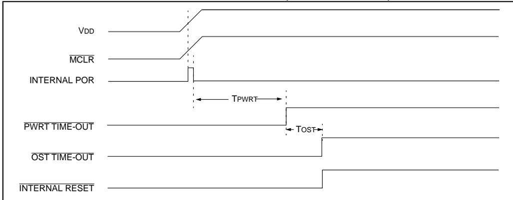
**FIGURE 11-8: TIME-OUT SEQUENCE ON POWER-UP ( $\overline{\text{MCLR}}$  NOT TIED TO  $V_{\text{DD}}$ ): CASE 1**
