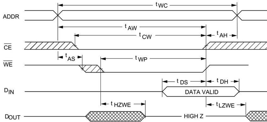
**Write Cycle No. 2 (Chip Enable Controlled)**
